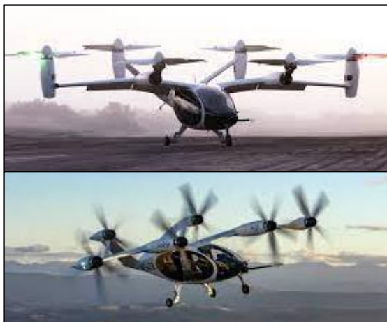
Figure 1. Joby S4 transitioning eVTOL aircraft at take off (top) and in forward flight.
